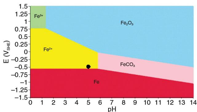
**FIGURE 2.** Example Pourbaix diagram for an Fe-H<sub>2</sub>O-CO<sub>2</sub> system with a system pH of 5.0 and a corrosion potential of -0.5 V.
